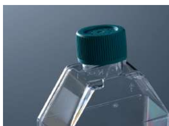
Vent caps with 0.22 um hydrophobic filters to ensure gas exchange without contamination
