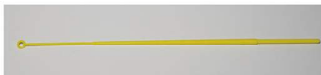
10 \mu L Inoculating loop
