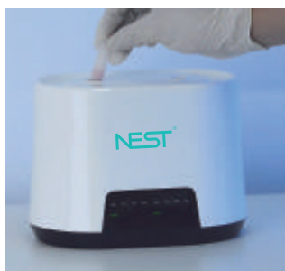
02 Insert the cryogenic tube into the hole
