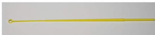
10 \mu L Inoculating loop
